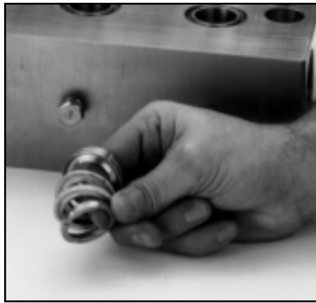
6811, 6821, 6831, 6841 Inlet Manifold and order of Packings
