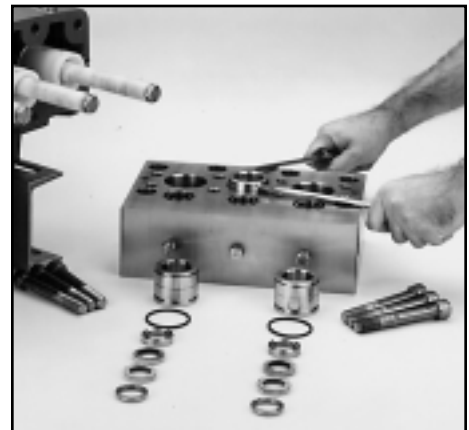
6811, 6821, 6841 Inlet Manifold and V-Packing Cylinder
