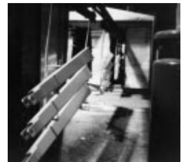
This conveyor load of parts has been treated with acid, thoroughly rinsed, dried and is now heading for the paint booth.
