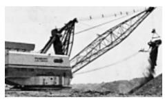
On this drag line, high pressure water removes daily accumulations of mud and/or coal dust from stairtreads, radiators etc. to allow efficient and safer operations.
